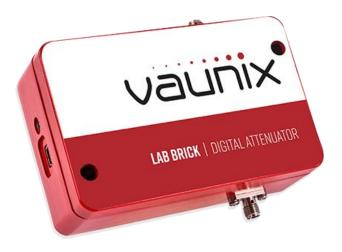
The Lab Brick LDA series of Digital Attenuators bring affordability, functionality, reliability and simplicity to the microwave test bench. The LDA products range from 10 MHz to 40 GHz with input level tolerance to 2 Watts and step size as small as 0.1 dB.
