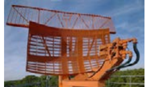
Sum-Difference Antennas are mounted to the larger Directional Antenna to generate beams that send pulses or coded interrogations.
