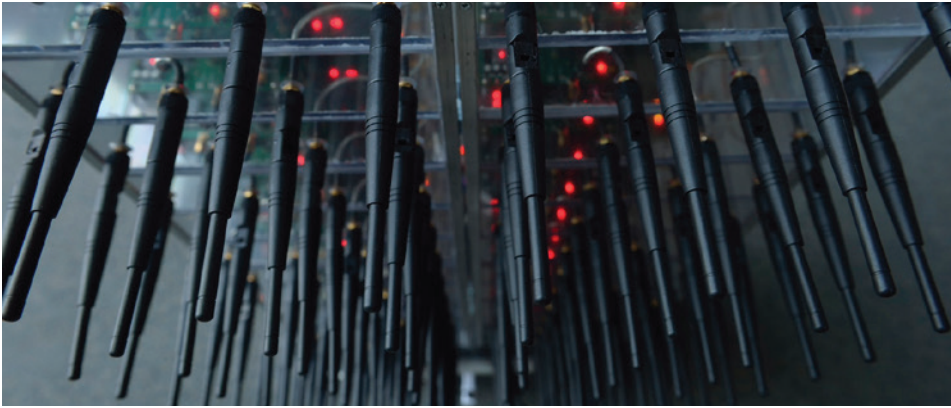
Massive MIMO test bed set-up.
