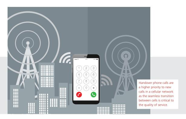
A handover, or handoff, occurs when an outgoing cellular connection is transferred from one cell to an adjacent cell while the user equipment is moving through the network coverage area.
